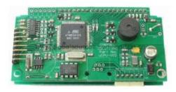
Next, move on to the circuit boards. Are they properly seated? Is there dust or spills on them? Are there signs of heat build-up? Are the components secure on the boards? Correct problems as you find them. You might look over the solder connections on the boards to be sure that there are no "cold" joints from previous repairs. You might also want to clean the connectors with a pencil eraser. Take note of any prior repairs: They are clues to current problems.
