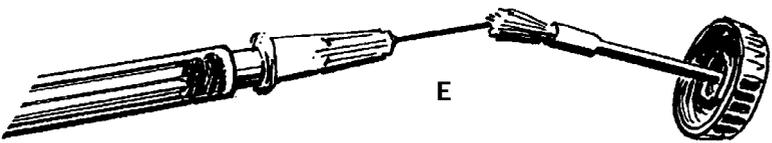
E. Moisten the tip of the needle with a small drop of soldering flux. Do not overfill the canula of the needle with the soldering flux. One should avoid the capillary action. This can be done by closing off the cone of the 16 or 18 G. needle. Put a 1 cc. syringe on the needle, the plunger should be on 0. There should be no air chamber present in the syringe as the flux will tend to reflux inside the needle, which will solder a large part of the lumen.
