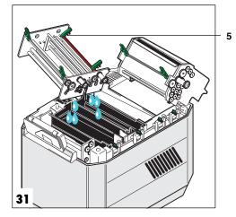
Remove roller packets for water (6) and developer/fixer (5); tilt sideways to allow chemicals to drain off
