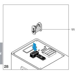
• Place the adapter (11), arrow downwards, into the loading slot.
