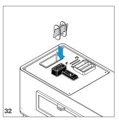
• Place the adapter vertically into the loading slot. The film edges must no be allowed to touch the shaft sides.
