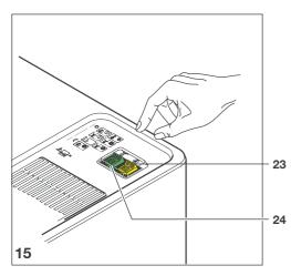
Check that the local supply voltage of the mains supply socket is identical to the voltage information on the model identification plate of the appliance.
