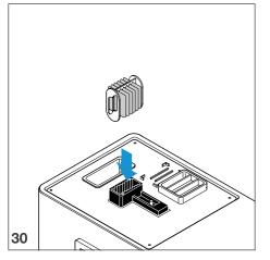
• Place the adapter vertically into the loading slot.
