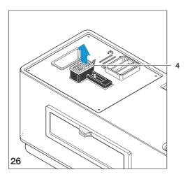
• Remove the cover (4) to the loading slot.
