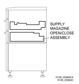
[1] Remove the SUPPLY MAGAZINE OPEN/ CLOSE ASSEMBLY with separation unit. If necessary, see the procedure on Page 2–42.
