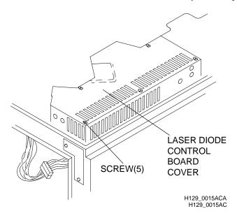
[3] Loosen the 5 SCREWS and remove the LASER DIODE CONTROL BOARD COVER.
