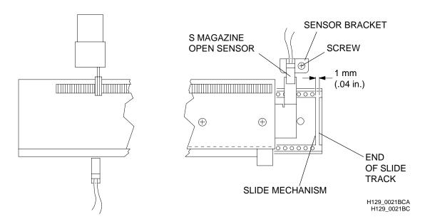
[7] Check that the distance between the END OF THE SLIDE TRACK and the SLIDE MECHANISM is 1 mm (0.04 in.).
