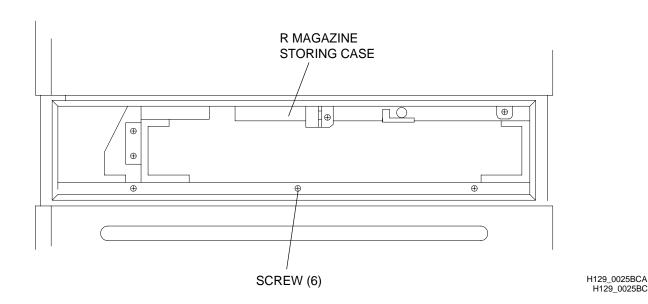
[9] Lift the R MAGAZINE STORING CASE and move it toward the front of the LASER PRINTER.
