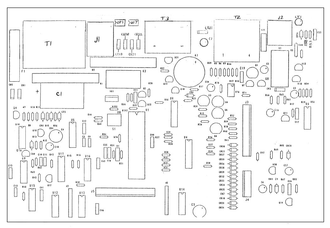
Component Layout for Timer/Driver PCBA (Summit Part No. 02249-002 Rev. C)
