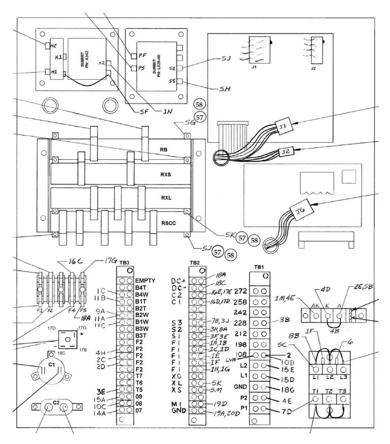
A323 ELECTRICAL CHASSIS for 325 generators
