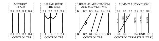
Note: Remove jumper clip across B1T and B2T on TB3 when connecting "table" bucky, or B1W and B2W on TB3 when connecting "wall" bucky.
