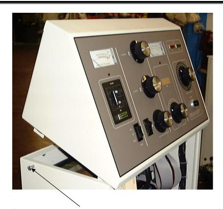
5. From the inside of the control, remove the two thumbscrews and washers from front panel being careful not to drop them into the cabinet.
