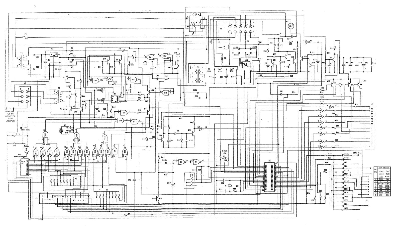
Schematic for Timer/Driver PCBA (Summit Part No. 02249-003 Rev. C)
