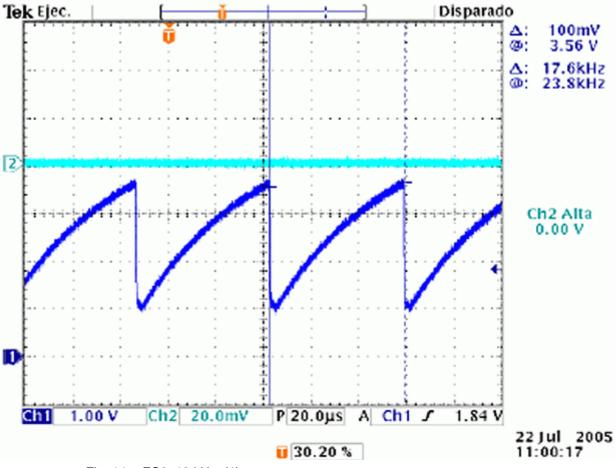
• If this is not the case, adjust P4 to 18 kHz  $\pm$  0.5 kHz.
