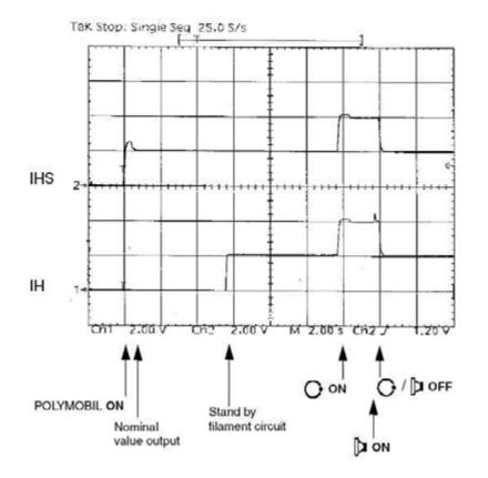
• Release an exposure with the default values 60 kV, 10 mAs.
