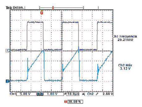
*Fig. 22:* D952\_FR1\_IC\_approx 27 kHz The capacitor charging frequency is approx. 27 kHz and cannot be adjusted.
