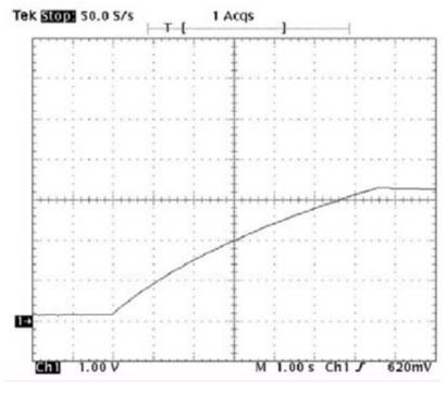
Fig. 23: Uc\_time\_ D916 test point "VC" (1V  $\triangleq$  100 V)
