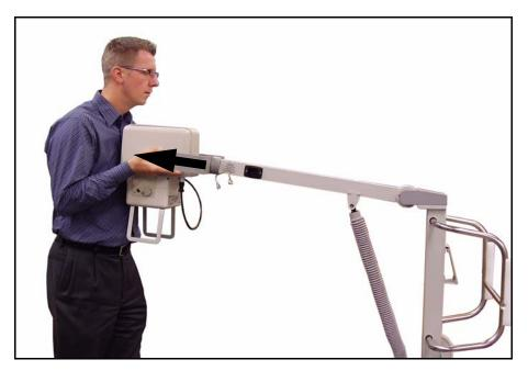
Figure 6-13. X-Ray Head Removal
