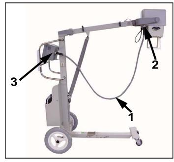
**17** Connect interconnect cable (1 in Figure 2-13). Female end to X-ray head (2) and male end to control console (3).
