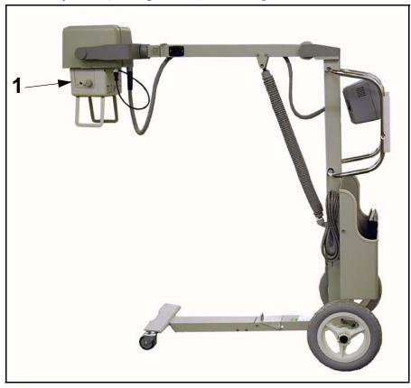
6 Turn X-ray head (1 in Figure 3-16) so that it points down.
