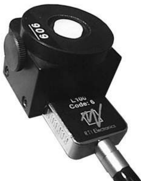
The Lux adapter with its cosine diffuser
