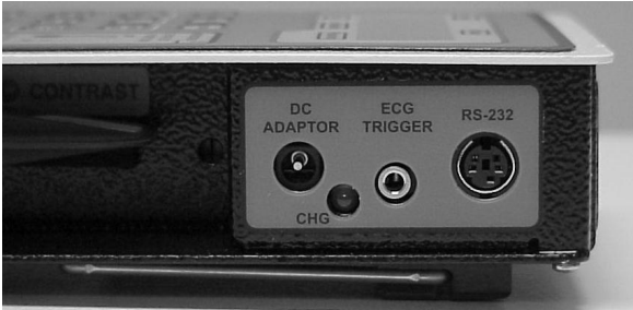
Figure 2 - Oxitest Plus 7 Side Panel
