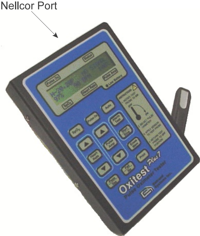
Figure 3 - Oxitest Plus 7 Front Panel
