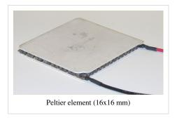
Thermoelectric junctions are generally only around 5-10% as efficient as the ideal refrigerator (Carnot cycle), compared with 40-60% achieved by conventional compression cycle systems (reverse Rankine systems using compression/expansion). Due to the relatively low efficiency, thermoelectric cooling is generally only used in environments where the solid state nature (no moving parts, maintenance-free, compact size) outweighs pure efficiency.
