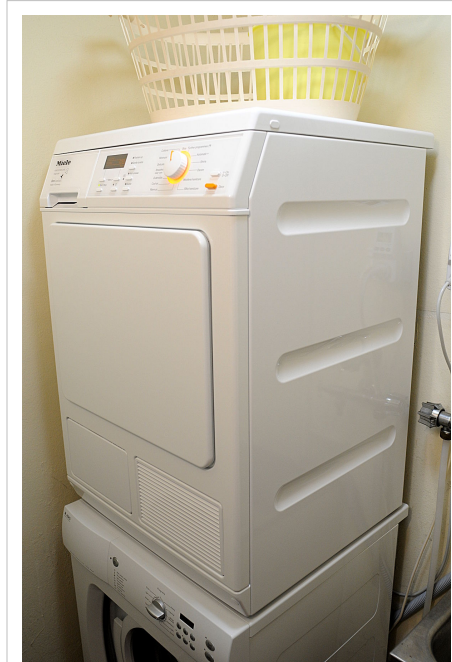
A closed cycle heat pump clothes dryer, using a heat pump to dehumidify the process air. Such dryers typically use less than half the energy per load of a condenser dryer.
