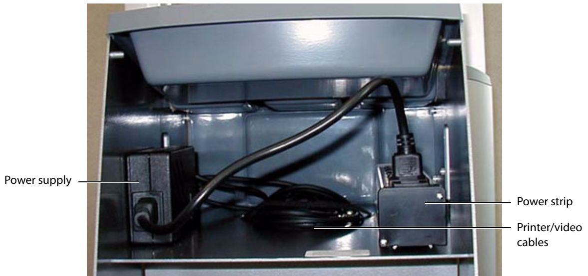
Figure 9.14 Mobile Docking System Power Supply
