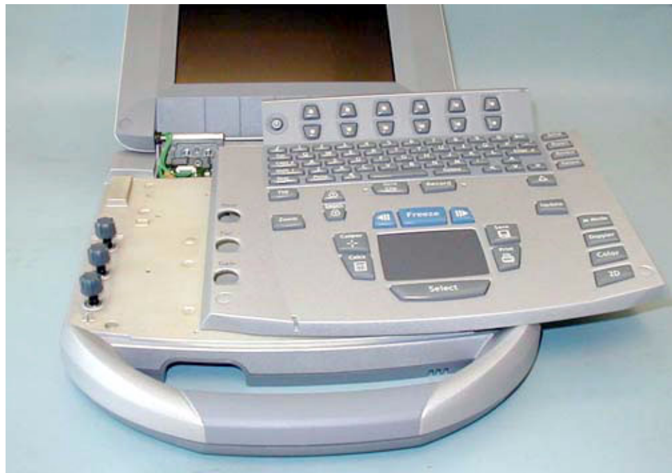
Figure 7.3 Control Panel Removal
