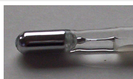
Closeup of a maximum thermometer. The break in the column of mercury is visible.
