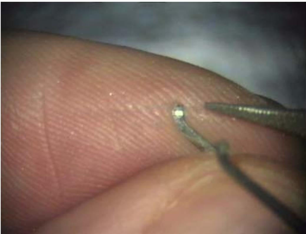
5. Make a groove on the other leg of the forceps at the same distance from the tip as on the first side.
