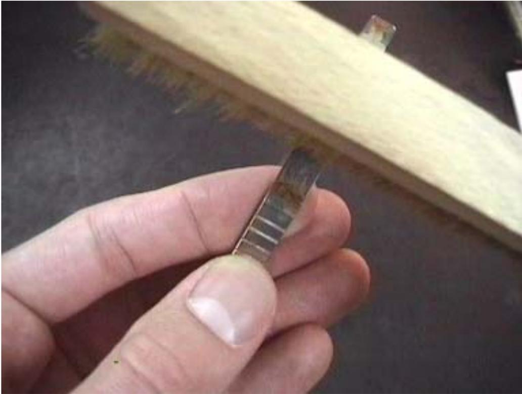
4. Do not use the brush on the working part of the instrument.
