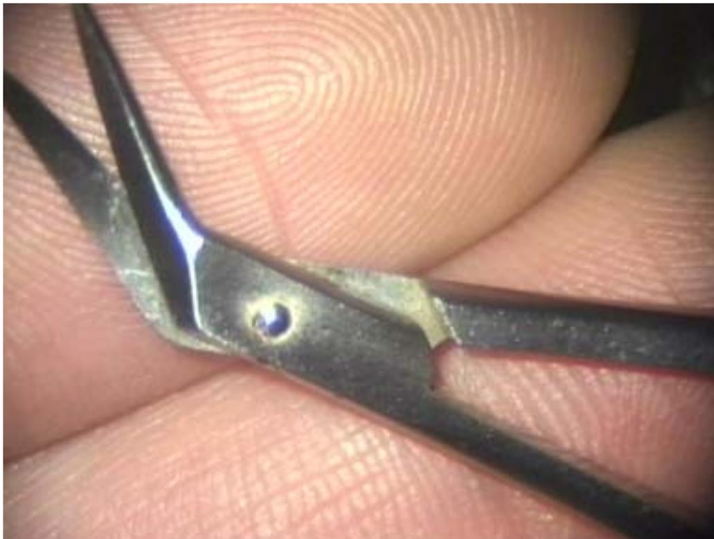
5. Open the lock of the instrument to make the joint accessible. Rotate the male part, so it can slip out of the female part. Do not use force to open the lock, since that might damage it.
