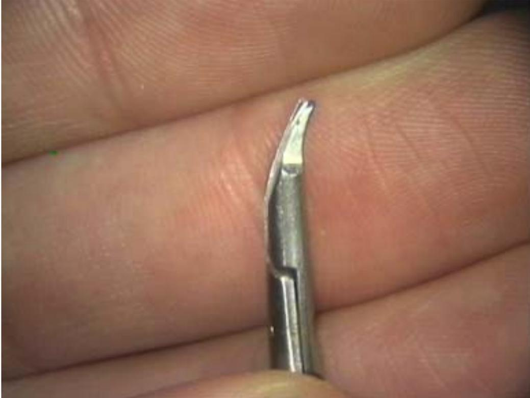
2. Rebend the bend side carefully, using a pair of flat tipped pliers. Do not use too much force.
