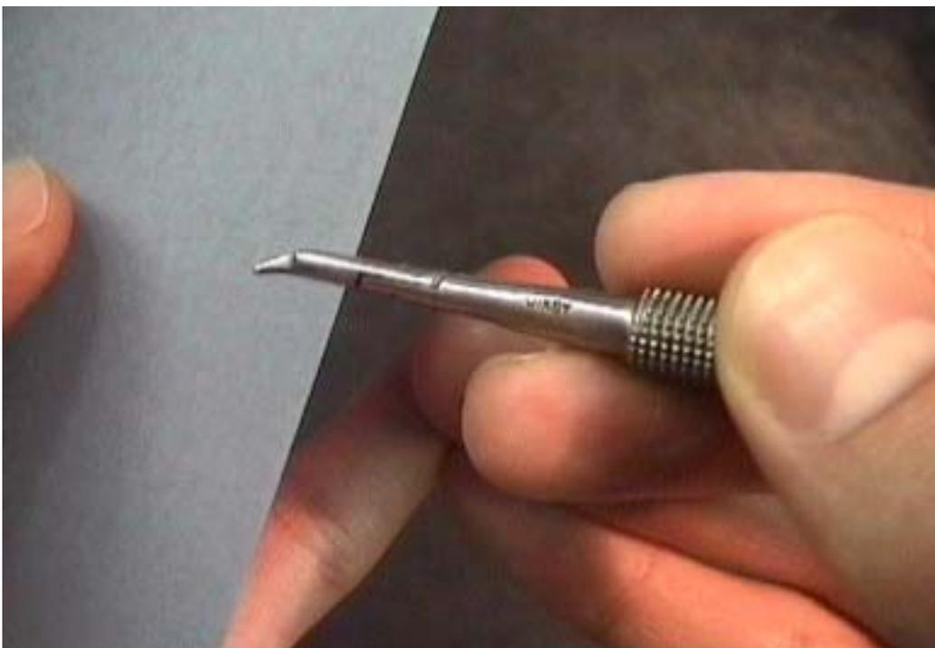
2. First polish one side, by moving the needle holders gently along the edge of the paper.
