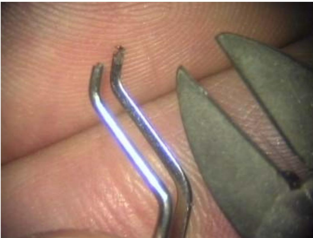
2. Smoothen both tips with a triangular file. Hold the tips of the forceps between thumb and index finger, this way the file cannot slip away.
