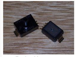
silicon piezoresistive pressure sensors
