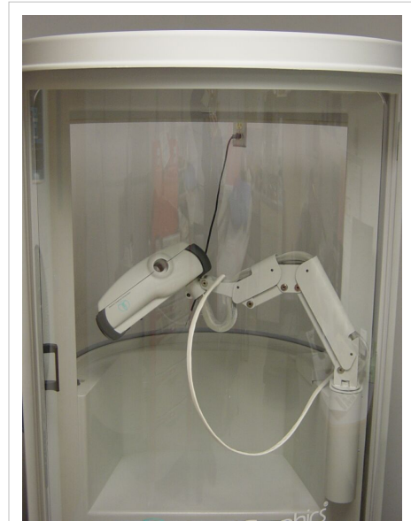
Plethysmograph or "body box" used in lung measurements.
