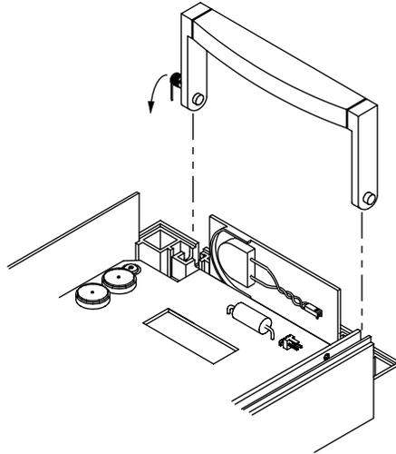
**Figure 6-7: Installing the Handle**
