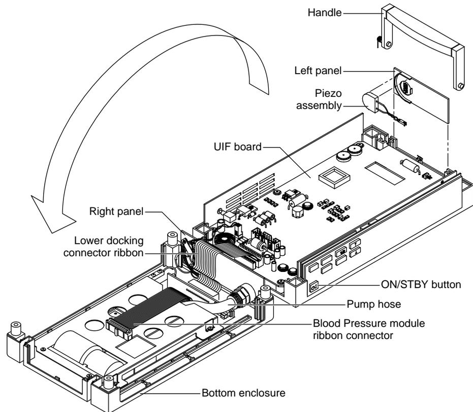
Figure 6-3: Separating the Monitor and Disconnecting the Cables
