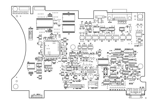
Figure 11-13 UIF PCB Parts Locator Diagram
