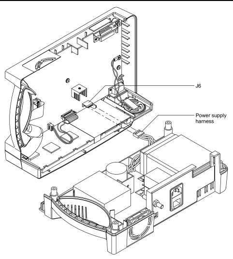
Figure 6-3: Separating Case Halves
