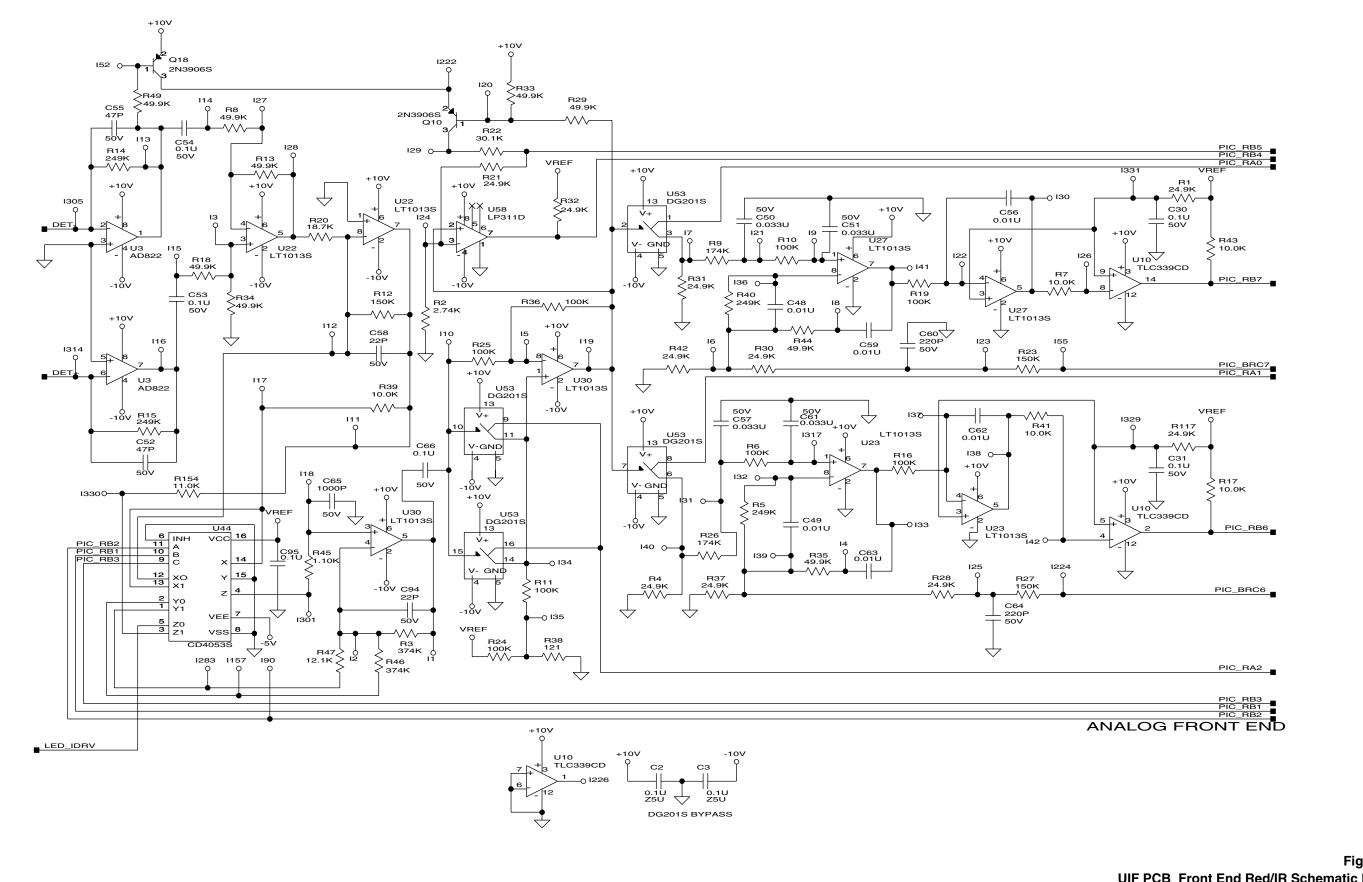
Figure 11-3 UIF PCB Front End Red/IR Schematic Diagram
