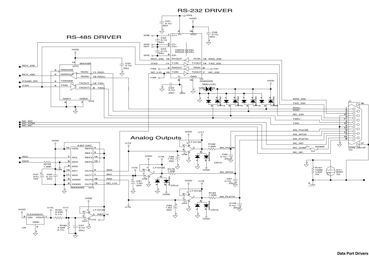
Figure 11-7 Data Port Drivers Schematic Diagram
