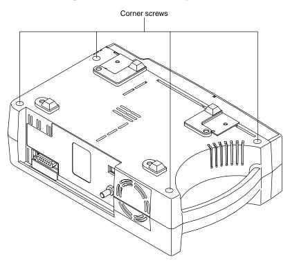
Figure 6-2: NPB-295 Corner Screws
