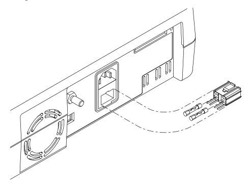
Figure 6-1: Fuse Removal
