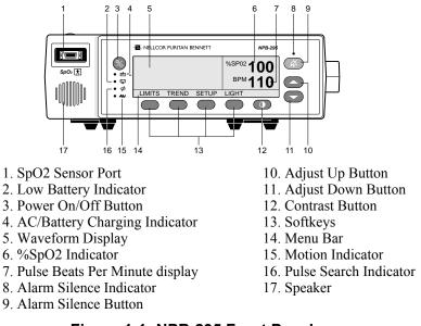
Figure 1-1: NPB-295 Front Panel
