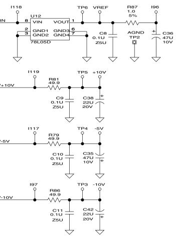
Figure 11-5 Front End Power Supply Schematic Diagram
