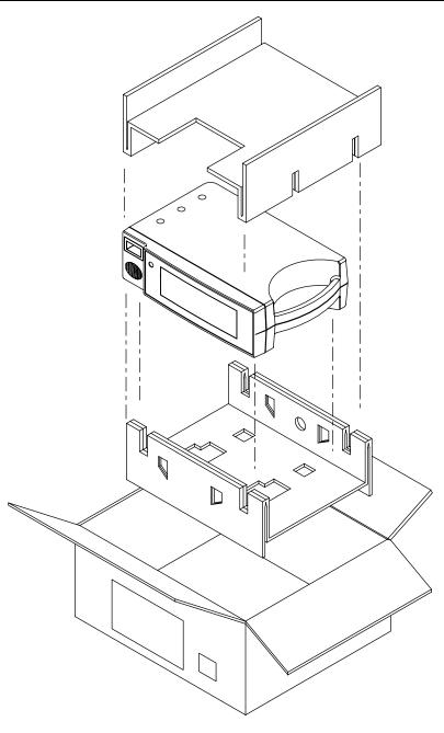
Figure 8-1: Repacking the NPB-295
