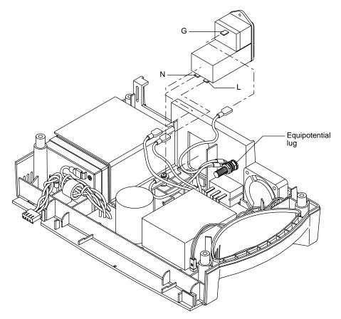
Figure 6-5: Power Entry Module
