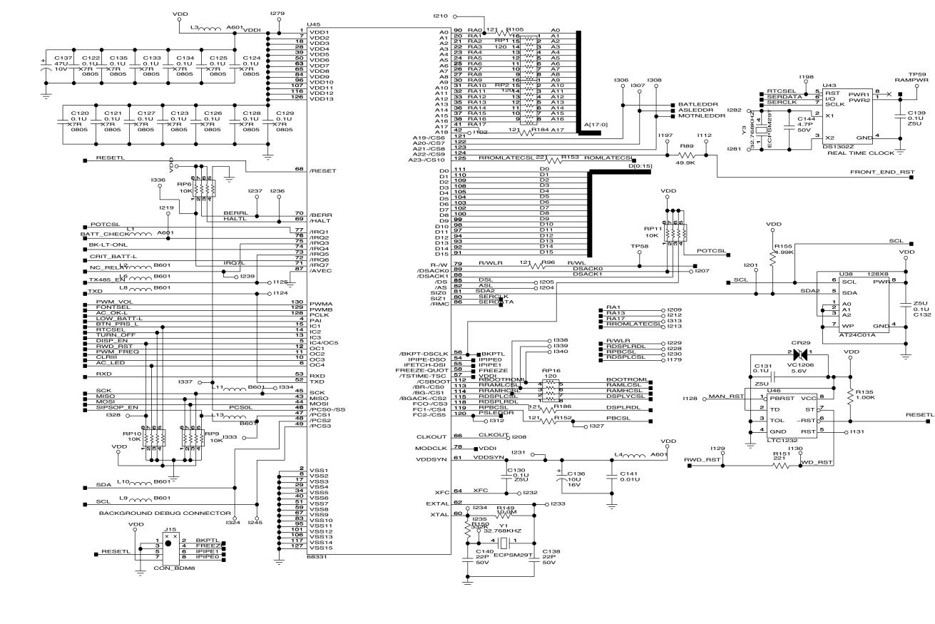
Figure 11-8 CPU Core Schematic Diagram A
