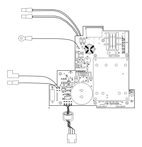
Figure 11-15 Power Supply Parts Locator Diagram
