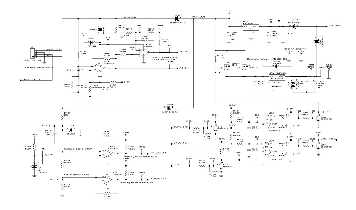
Figure 11-11 UIF PCB Power Supply Schematic Diagram B
