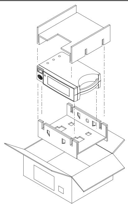
Figure 8-1: Repacking the NPB-290
