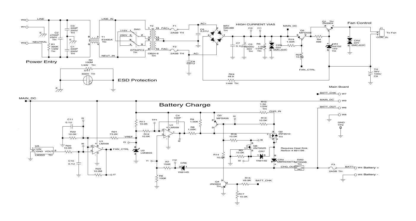
Figure 11-14 Power Supply Schematic Diagram
