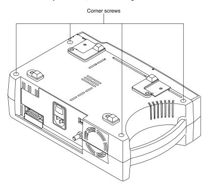
Figure 6-2: NPB-290 Corner Screws
