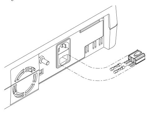
Figure 6-1: Fuse Removal
