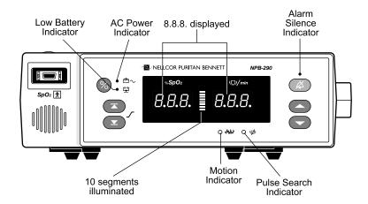
Figure 3-2: Power-On Self-Test Display
