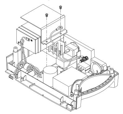
Figure 6-4: Battery Removal
