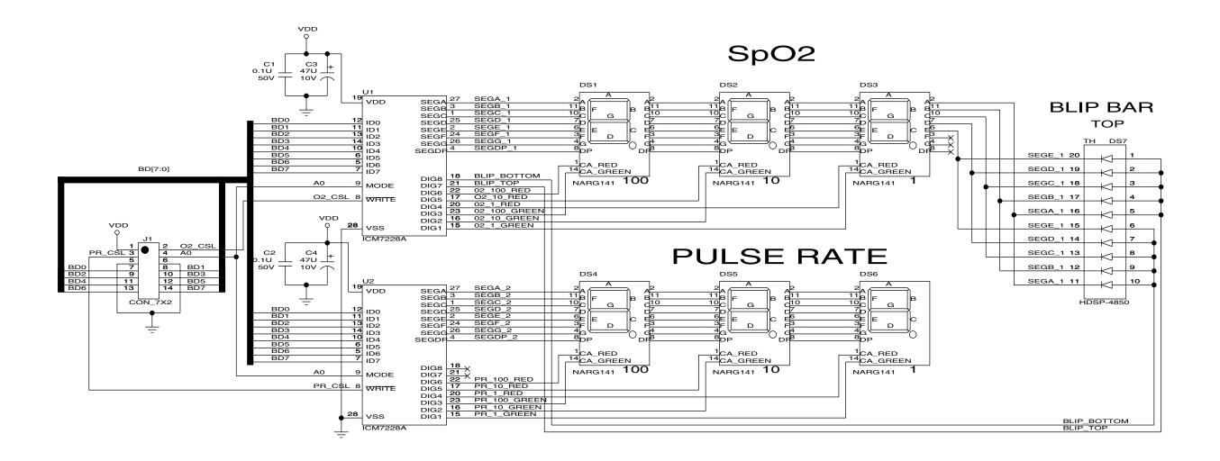
Figure 11-16 Display PCB Schematic Diagram
