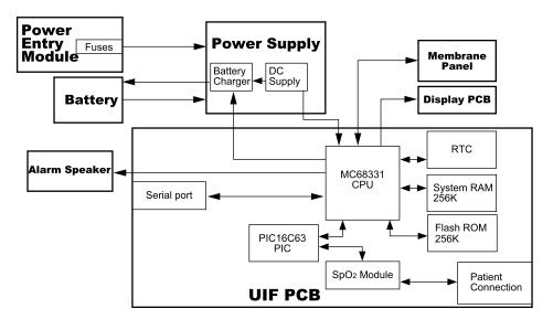
Figure 11-2: NPB-290 Functional Block Diagram
