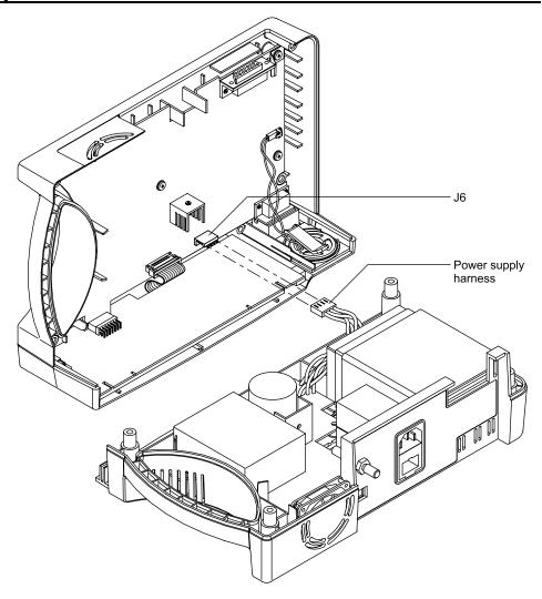
Figure 6-3: Separating Case Halves
