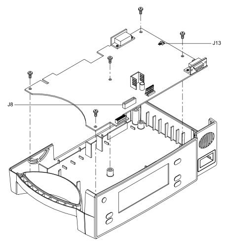
Figure 6-9: User Interface PCB
