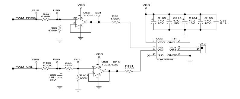
Figure 11-10 Speaker Driver Schematic Diagram A
