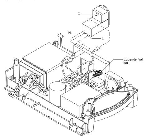
Figure 6-5: Power Entry Module
