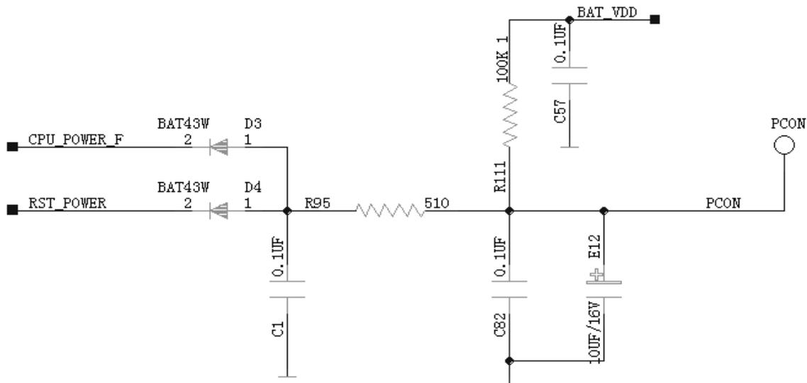
Fig 2-7 Switch On Circuit
