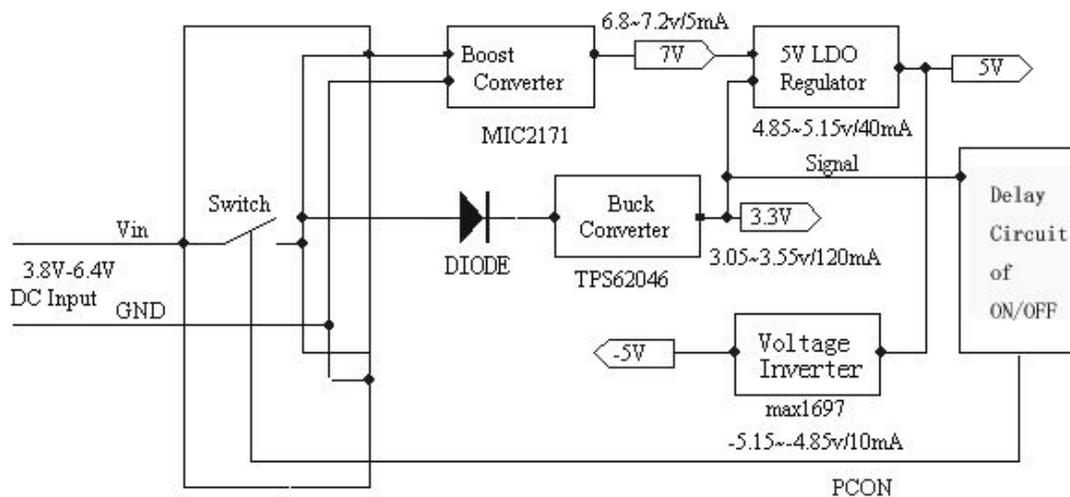
Fig 2-10 Power Supply Circuit Block Diagram
