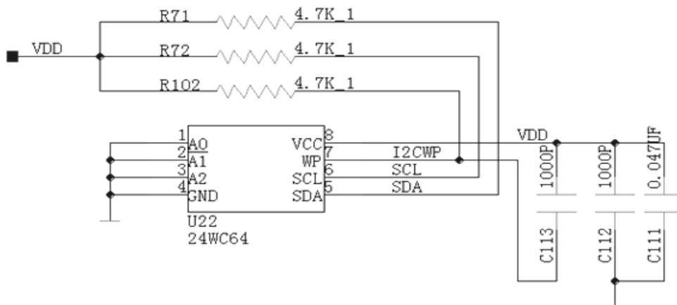
Fig 2-3 Data Storage Circuit
