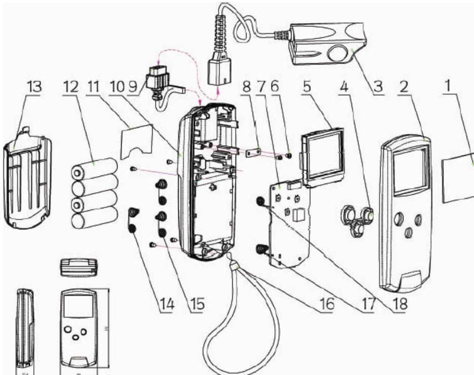
Fig 4-1 Pulse Oximeter Explosive diagram (0850-30-30752)
