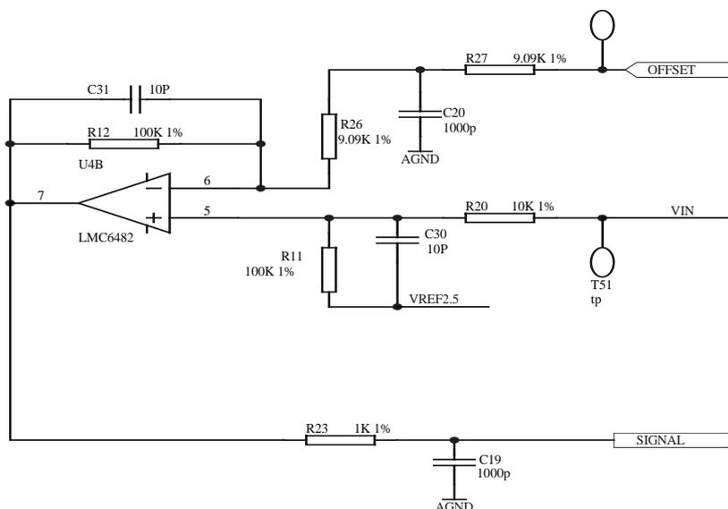
Fig 2-5 Voltage Shift Circuit
