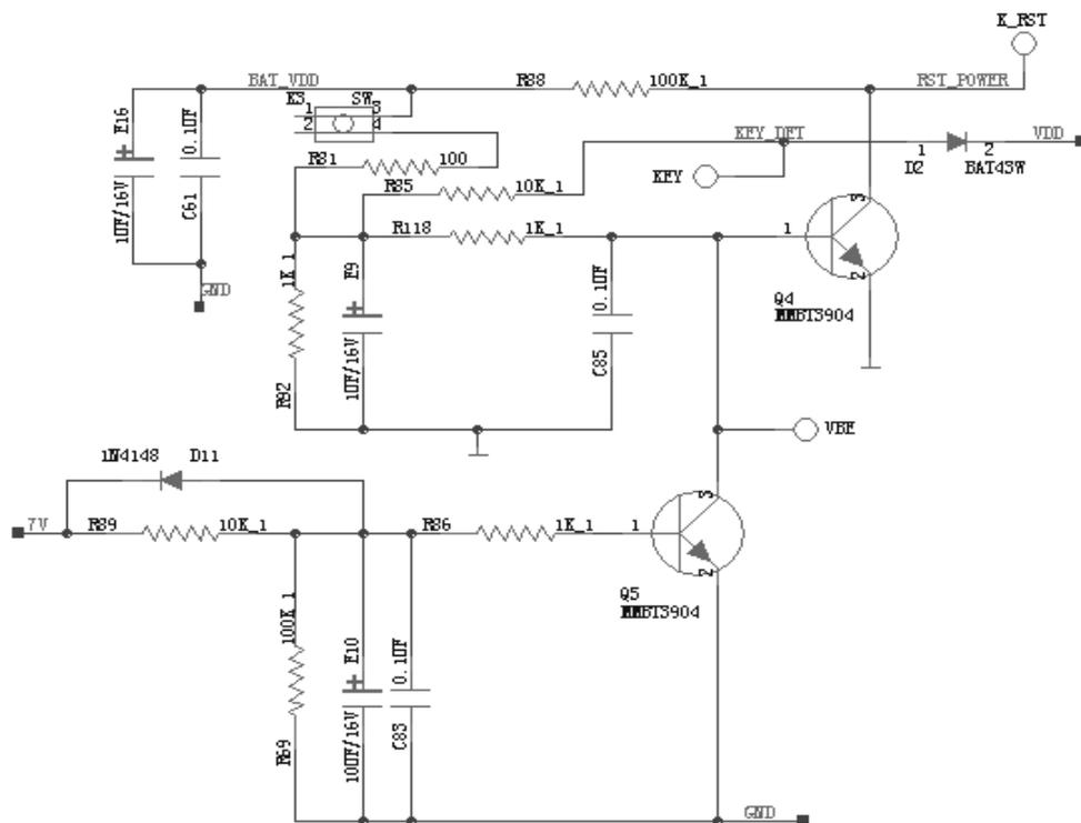
Fig 2-6 Delay Circuit Block
