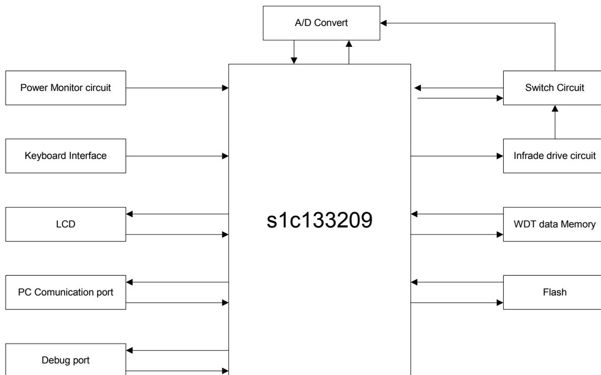
Fig 2-1 Pulse oximeter Block Diagram
