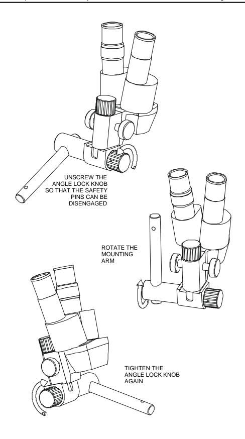
Figure 12b Changing the assistant microscope configuration
