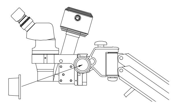
Figure 9 Inserting the focus control covers
