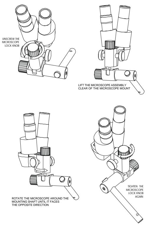
Figure 12a Changing the assistant microscope configuration
