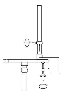
Figure 3 Attaching the clamp to the mounting surface
