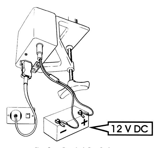
Figure 7 Connecting the Power Supply
