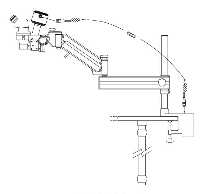
Figure 6 Connecting the lamphouse cable
