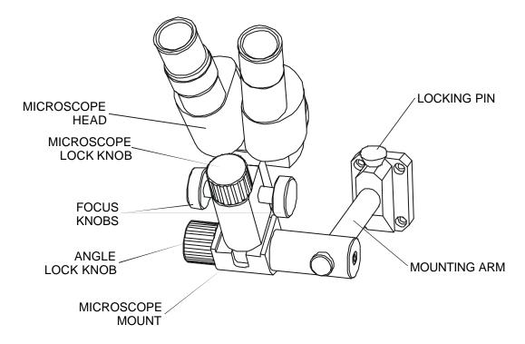
Figure 11 Binocular Assistant Microscope
