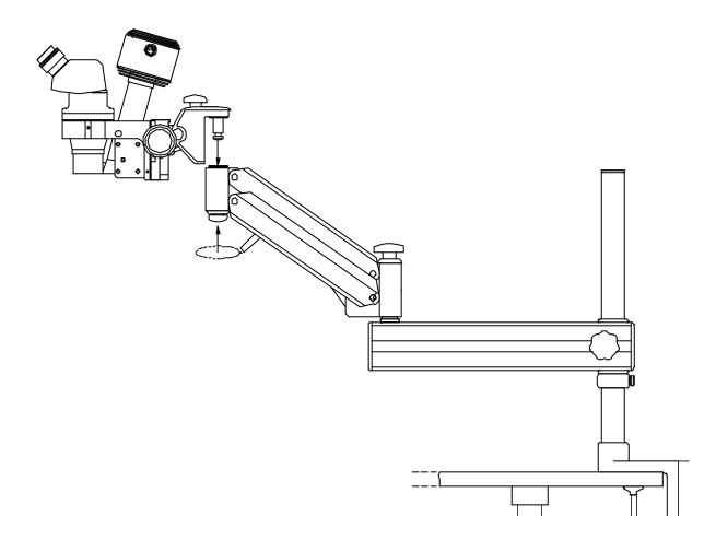
Figure 5 Attaching the microscope assembly
