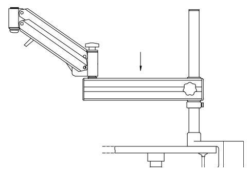
Figure 4 Attaching the arm assembly
