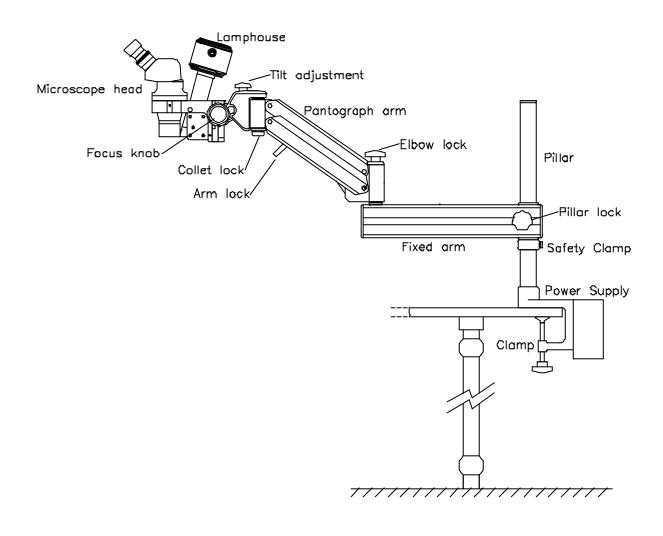
Figure 1 Scan Optics SO-161 Ophthalmic Microscope
