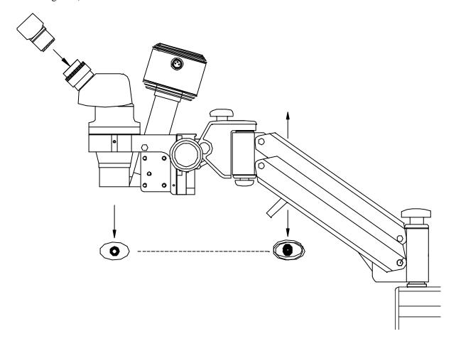
Figure 8 Inserting the eyepieces and rough focusing
