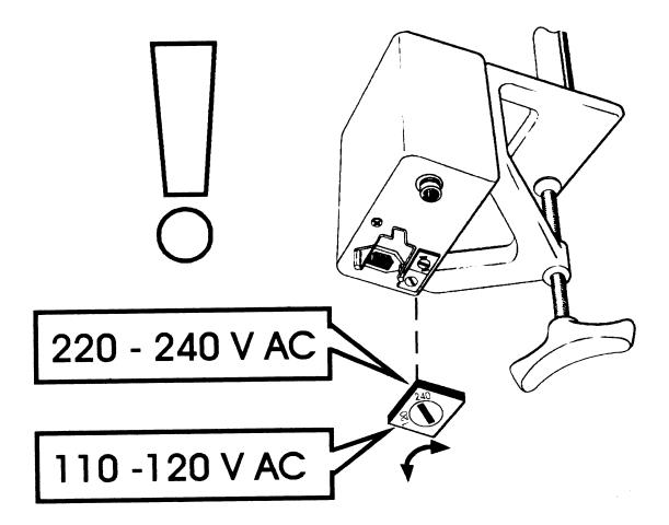
Figure 2 Setting the mains voltage
