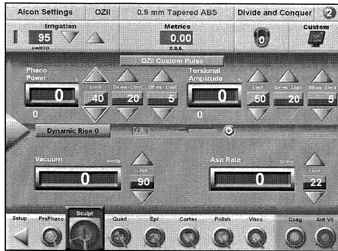
Figure 2-73 The OZil ® Custom Pulse Surgery Screen - In this mode of operation there is a repeating SEQUENCE of events as follows: phaco power, then an off-time, ultrasonic oscillations, then an off-time. The Phaco Power Limit and Torsional Amplitude Limit set the strength of each. The duration of each is set with the On ms - Limit and Off ms - Limit settings.
