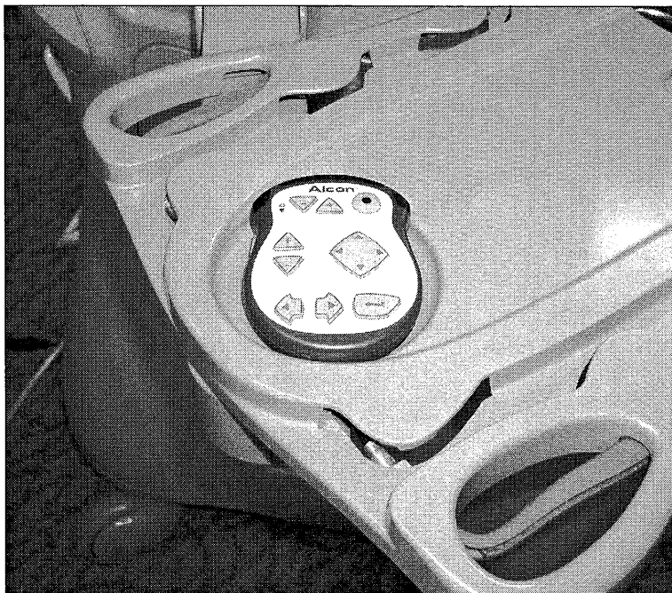
Figure 2-9 The Remote Control - The remote control fits securely in its tray assembly receptacle and allows rotation in any orientation. The sterile tray support cover is then draped over the remote and tray.
