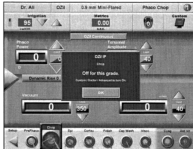
Figure 2-76 OZil ® IP Dialog - This dialog shows that OZil ® IP feature is turned Off for this cataract grade. To turn it On for this cataract grade, it must first be enabled in the Custom / Doctor / Advanced window.
