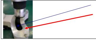
Please add some silicon oil or grease. Grease lightly to inside of sliding position. Do not grease too much on the top of the sliding place.
