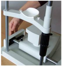
Mount the camera head to the base using two Allen screws.
