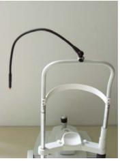
Connect the USB cable\* to a port of the PC as power supply for the external fixation lamp.
