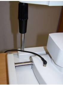
Connect the cable for R/L detection to the power supply.
