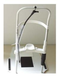
Insert the base of the fixation light into the protruding plug-in on top of the head rest. Screw on the external fixation light.
