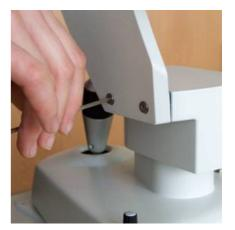
Connect the cable for right/left (R/L) detection to the camera base.
