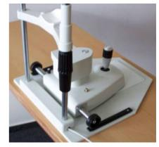
Fit one of the protective covers over the gear rail at the side and slide the base forward up to the stop.
