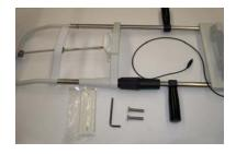
Fasten the chin rest to the table using 2 Allen screws (see drilling jig and corresponding holes in the table).
