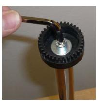
Slide the guide rail through the base. Screw on the gear again.
