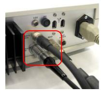
Connect the foot switch to the socket "foot switch".
