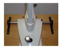
Fit one of the protective covers on the mounted gear rail at the side and slide the base forward up to the stop.
