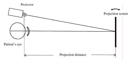
Figure 5-1: Direct projection (top view)
