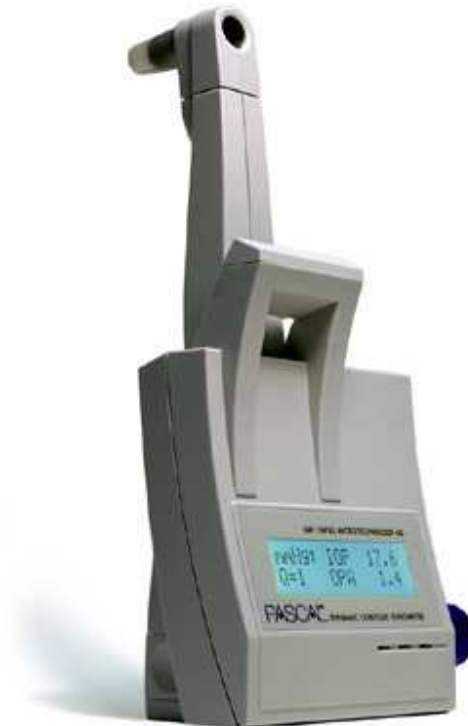
Fig. 10. The PASCAL® contoured piezoresistive sensor tip
