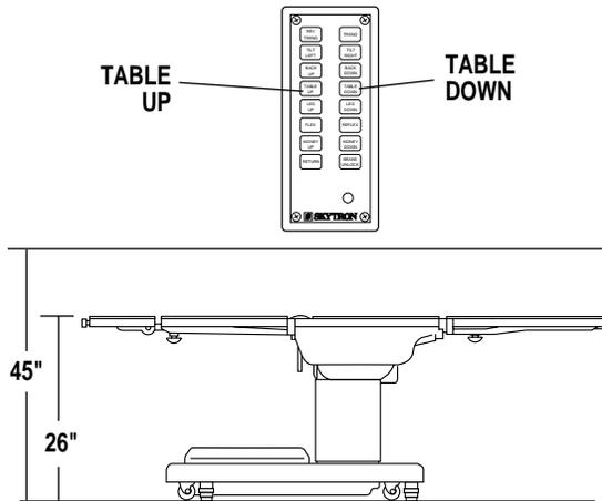
**Figure 3-8. Elevation Function**
