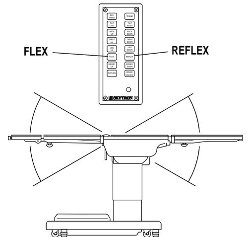
**Figure 3-10. Flex/Reflex Positioning**
