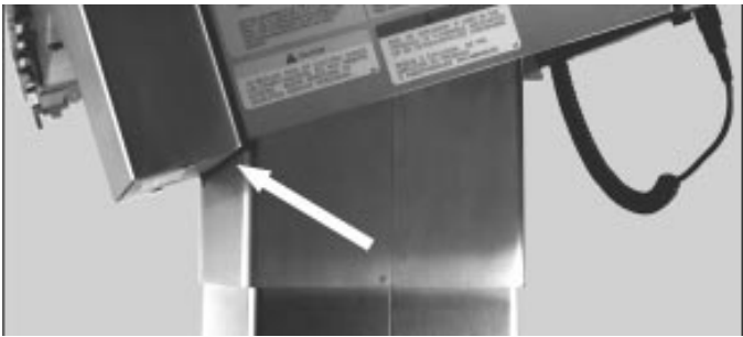
FIGURE 10 ..... Left Side Pinch Point
