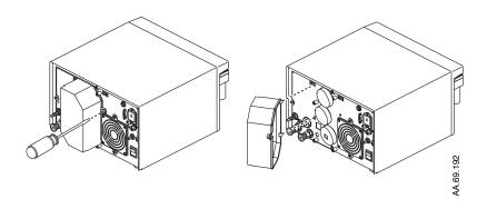
Figure 15-7 • Sensor cover removal and replacement
