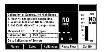
3. Push the control wheel to display the NO high range calibration menu. A display similar to figure 10-9 appears.
