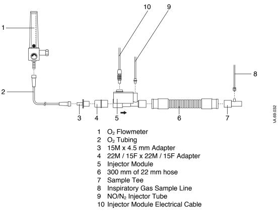
Figure 10-2 • Circuit connections for purge and performance test
