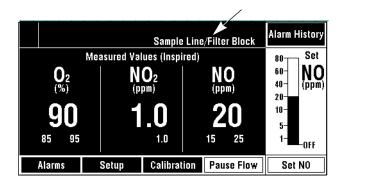
*Figure* 7-3 • Low priority alarm message shown in low priority alarm location
