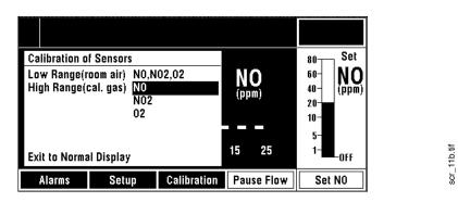
*Figure 10-8* • Calibration menu - high range NO sensor calibration option highlighted
