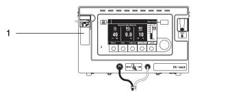
1. Fluid Trap Filter Cartridge
