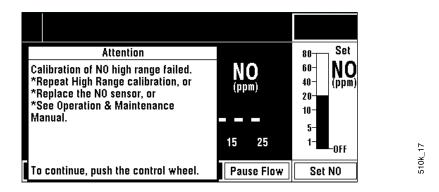
*Figure 4-10* • High range calibration menu example - NO high range calibration failed
