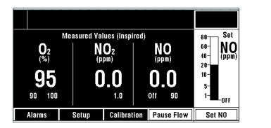
Figure 6-14 • Set NO display - normal state, NO bargraph showing 20 ppm setting
