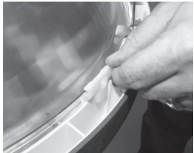
Figure 8-34. Lens Clip Removal
