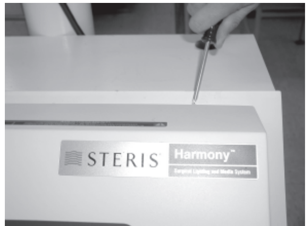
Figure 8-18. Loosen Screws at Top of Control Center Cover
