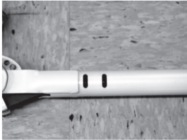
Figure 8-7. Monitor Spring Arm Tension Adjustment Access
