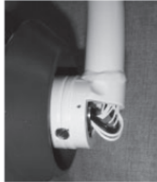
Figure 8-16. Ensure Looped Wires are Dressed Away from any Moving Parts.
