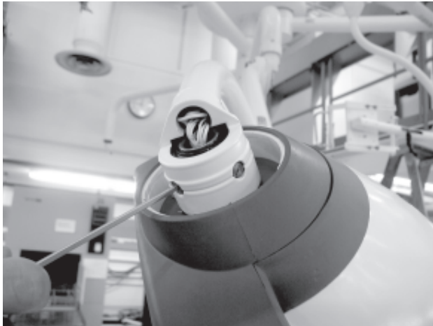
Figure 8-1. Adjust Lighthead/Yoke Brake Tension
