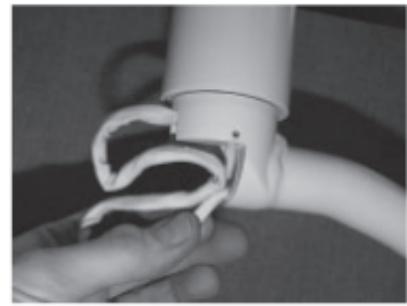
Figure 8-14. Fold Wiring into Loop
