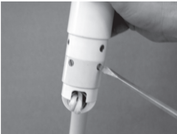
Figure 8-3. Adjust Spring Arm/Yoke Brake Tension
