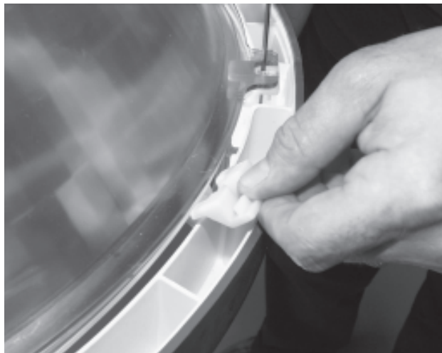
Figure 8-32. Lift Lens Using Spare Lens Clip
