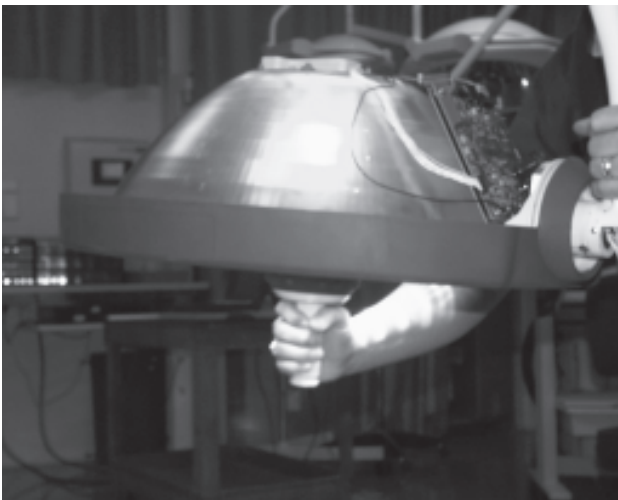
Figure 8-27. Reposition Lens Assembly Using Lighthouse
