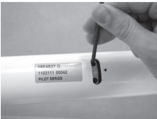
Figure 8-6. Adjust Spring Arm Tension
