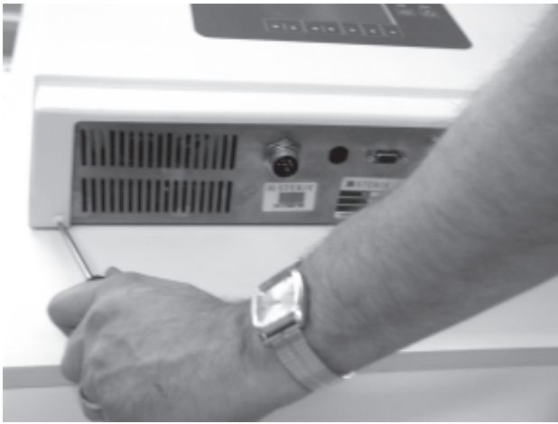
Figure 8-18. Remove Control Center Bottom Screws
