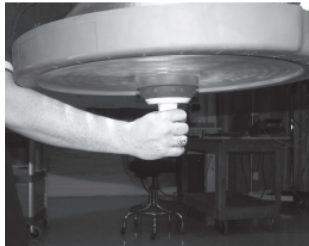
Figure 8-28. Rotate Lighthouse Handle to Check for Binding
