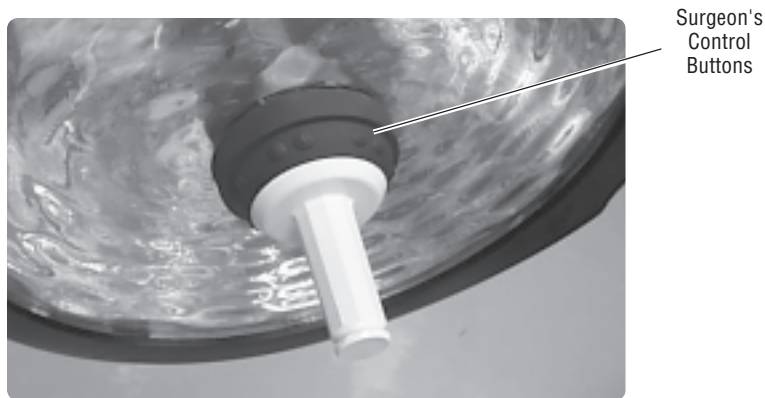
Figure 3-2. Lighthead Surgeon's Control Buttons (Harmony LA 500 Lighthead with Standard Handle Shown)
