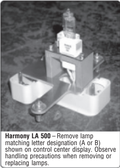
Figure 6-3. Lamp Replacement Procedure (Harmony LA 500 Lighthouse Shown)
