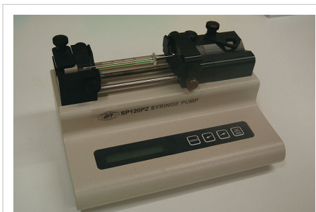
A syringe pump for laboratory use. World Precision Instruments (WPI) SP120PZ.
