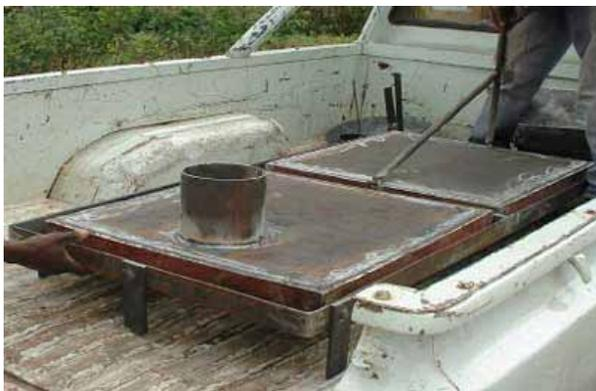
Photo 3: welded steel top with door and chimney spigot ready to be installed
