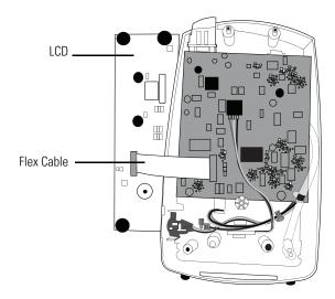
3. Remove the flex cable from the LCD and set the LCD aside.
