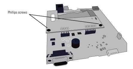
2. Remove the two phillips head screws and lift the Masimo adapter board straight up. There are four connectors on this board - two connect to the main PCB and the other two connect to the Masimo PCB.
