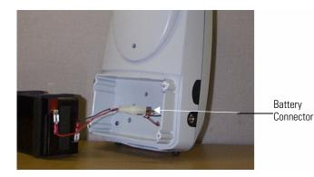
4. Slide the new battery completely into the compartment. Lay the connector on the battery. The relief pocket in the battery door purposely provides sufficient clearance for the battery connector.
