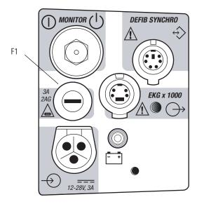
To remove the fuse, use a flat blade screwdriver to turn the fuse cover and release the fuse.
