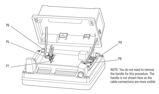
Detach the ribbon cable from the Rear Chassis (see below):
