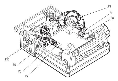
2. Torque the five screws securing the Interface Chassis to the Front Chassis to 6.65 to 7.35 in-lb (0.75 to 0.83 N-m).
