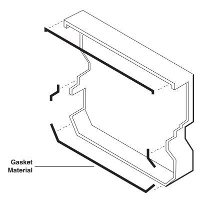
4. Set the Chassis onto the rear panel, confirming that the gaskets don't slip out of a channel and become pinched between the rear panel and the Chassis.
