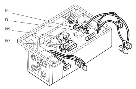
5. Remove the four screws securing the Recharger Board to the Rear Chassis. Note the screw passing through the pressure transducer is longer than the three that pass through the Board only.
