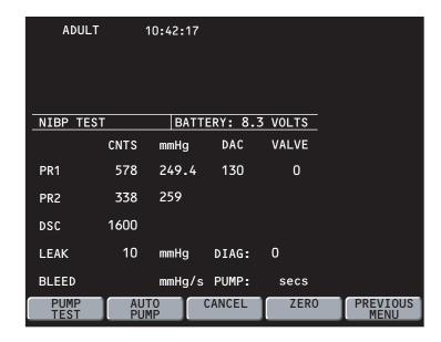
7. Manually reduce the pressure as indicated on the pressure meter to each of the levels shown in the following table, and check the displayed value of PR1 to be within the tolerance listed in the following table.
