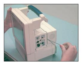
3. Slide the monitor forward until you can disconnect the battery pack cable from the monitor's power cable (see below). The battery pack should remain in the Expansion Module Chassis.
