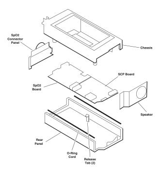
When closing the SpO<sub>2</sub> module, confirm that no O-ring gasket slips out of its channel and becomes pinched between the rear panel and the Chassis.
