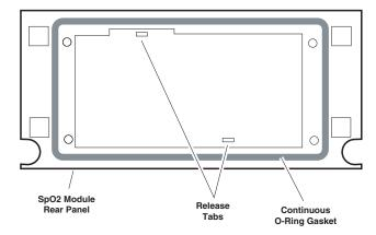
3. After the tabs allow the rear panel to be removed, separate the rear panel from the chassis.
