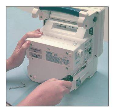
3. Separate the front panel from the Chassis, disconnecting the front panel cable from the Expansion Module button board.
