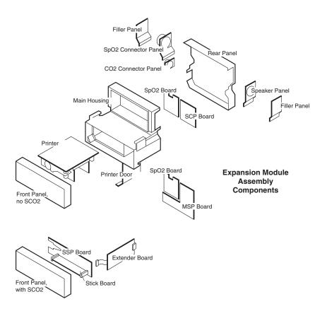
**Note** The Expansion Module does not need to be separated from the monitor to replace the Expansion Module front panel.
