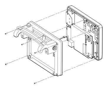
5. Remove the five screws fastening the Analog Board to the Front Chassis.
