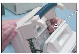
Disconnect tubing from pressure transducer
