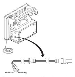
Connect the adapter cable to the monitor's dc input jack.
