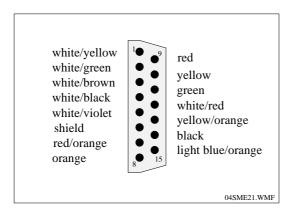
The configuration of the different ECG plugs which can be directly connected to the APPLICARD may be obtained on request.
