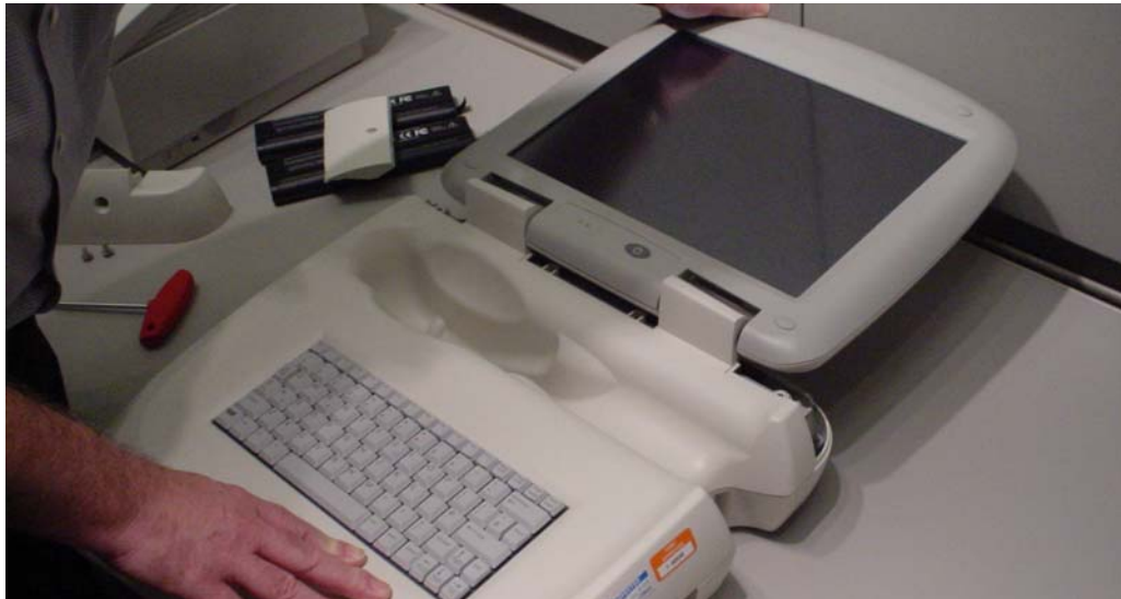
Figure 6-33 Rotating the Display Down
