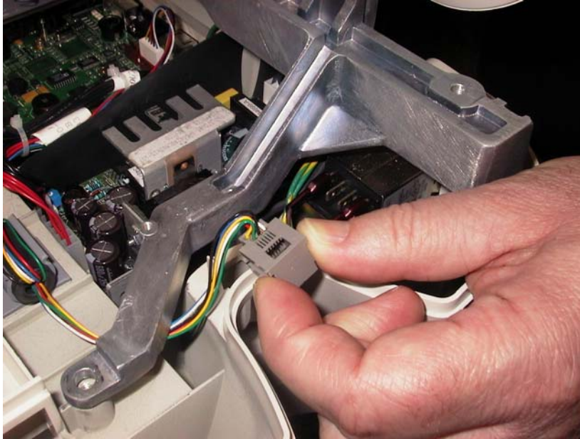
Figure 6-82 Removing the PIM Connector
