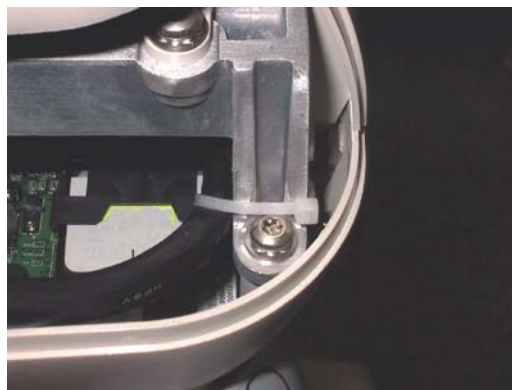
Figure 6-44 Location of the Tie Wrap For the Display
