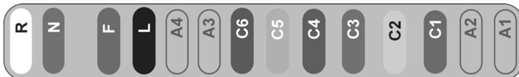
Figure 6-18 16-Lead IEC PIM IEC Lead Wire Labeling
