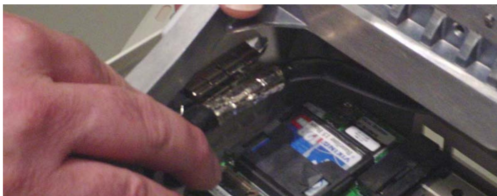
Figure 6-39 Removing Display Cable From Bracket
