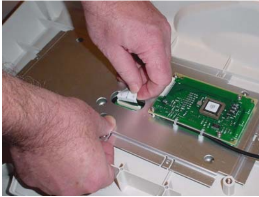
Figure 6-53 Disconnecting the Flex Cable
