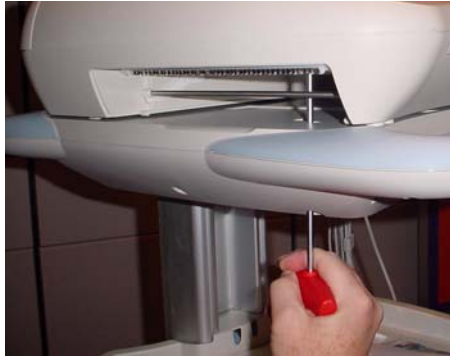
Removing screws with cardiograph on cart
