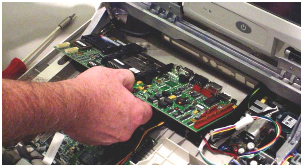
Figure 6-72 Lifting Out the Main Control Board
