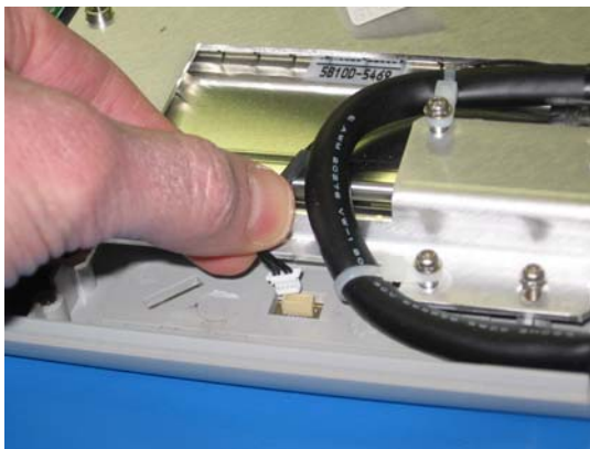
Figure 6-47 Disconnecting the On/Standby connector
