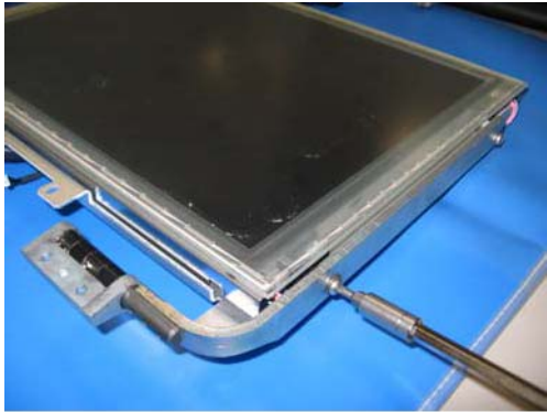
Figure 6-50 Removing the two M5 x 9mm screws
