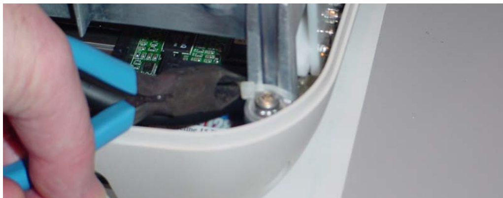
Figure 6-38 Cutting the Tie Wrap
