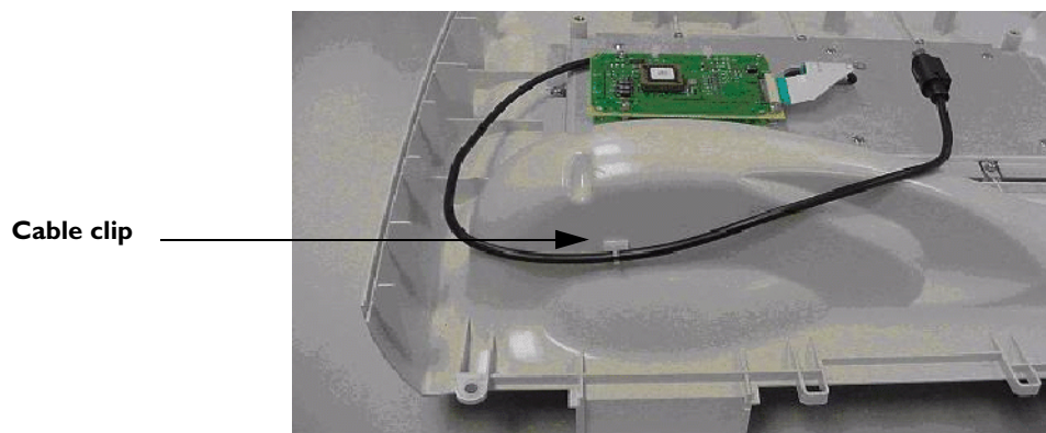
Figure 6-36 Keyboard Cable Routing
