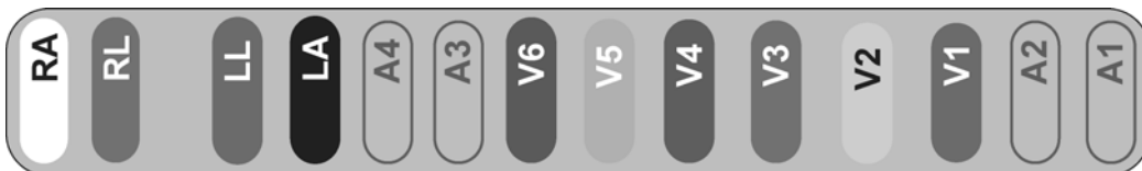
Figure 6-18 16-Lead IEC PIM IEC Lead Wire Labeling
