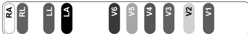
Figure 6-16 12-Lead PIM IEC Lead Wire Labeling
