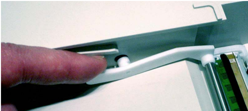
Figure 6-61 Removing the Paper Guide Bar
