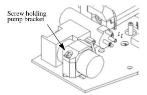
**Step 3** Gently disconnect the flow tubing attached to the Extension from the Pump.
