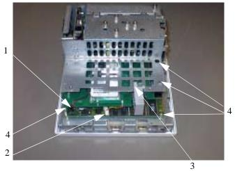
**Step 7** Remove the 4 System Board screws (4).
