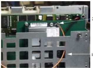
• Connect the free end of the antenna cable to the connector on the corner of the wireless LAN board (2, above).
