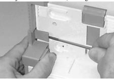
**Step 7** Lay the Monitor on its rear panel and pull out the two latches - there is one on each side of the Monitor Bezel.
