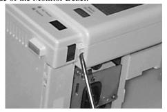
**Step 8** Stand the Monitor up again and gently lift the Monitor Bezel up and out. Gently let it rest in front of the Monitor. Be careful. It still has a cable attached.
