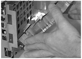
**Step 6** Unplug the backlight tube cables.
