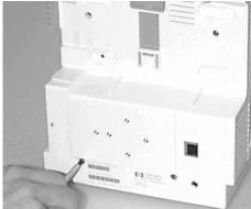
Step 12 Slide the chassis slowly out from the front of the housing (the battery compartment cover must be open), and lay the chassis on the Monitor Bezel For Monitors with a Wireless LAN Assembly: To avoid antenna damage, slide the chassis very carefully out from the front of the housing, disconnect the antenna cable and lay the chassis on the Monitor Bezel.
