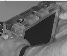
**Step 5** Lay the LCD display on a flat, scratch-free surface.
