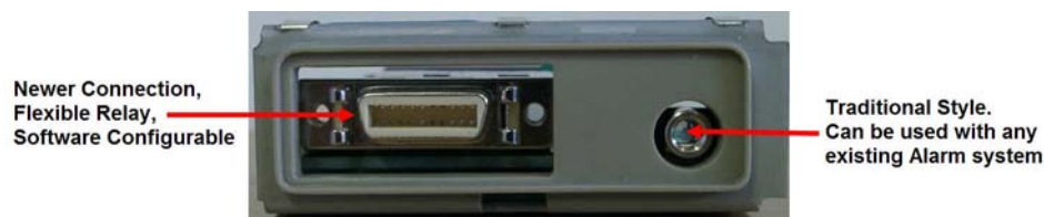
Flexible Nurse Call Relay Connections at Monitor
