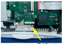
Black Spacer is attached to main board with one screw
