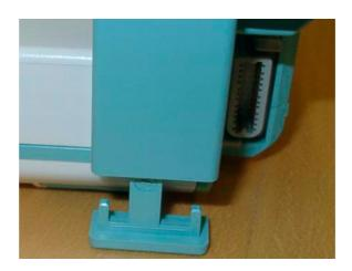
7 Lift part A upwards. It is fixed in a dovetail. Be careful with the MSL flex.
