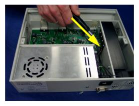
4 Lift the fan out of the battery conditioner housing.
