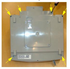
3 Remove the four screws securing the metal plate and lift it off.
