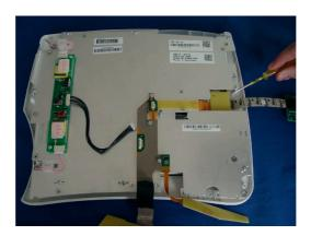
7 Unscrew the three screws and remove the flex panel adapter cable.
