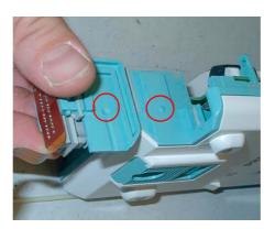
2 Lift up the flex connector carefully. Do not bend the connector pins on the main board.
