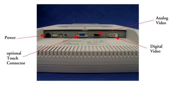
Figure 24 Connections M8033A
