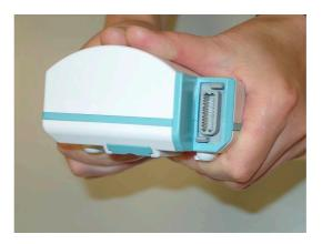
4 Holding the bottom cover firmly in place, slide the two long mounting pins completely back into the MMS. Make sure there is no gap between the top and bottom cover.
