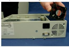
5 When replacing the fan make sure the connector is plugged in correctly as shown in the photograph below.
