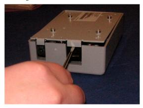
Turn the IIT box around and lift the top cover off completely. Then unplug the flex cable from the PCA board.
