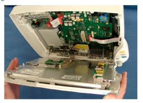
**Reassembly Note:** Make sure the metal sheet on the back of the display is inserted into the noses of the monitor rear housing when reassembling the two halves.
