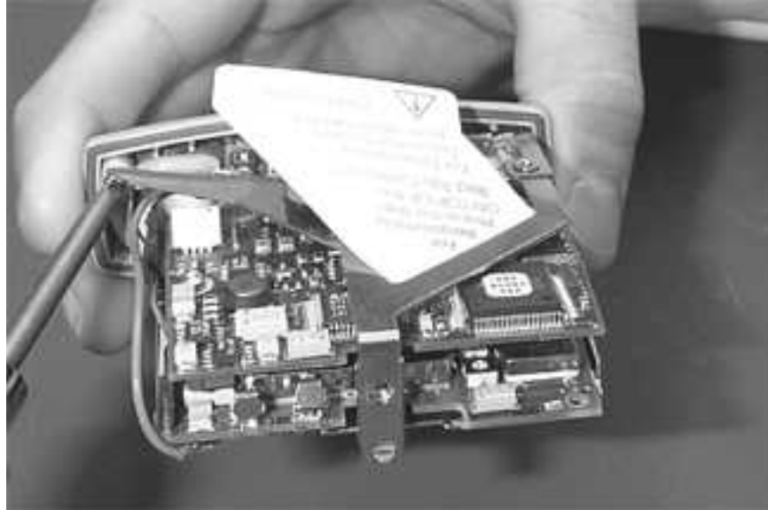
Figure 6-16 Secure the Main Cage Brace
