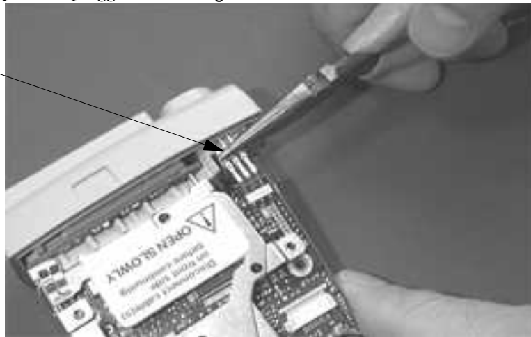
Figure 6-3 Hold the Lead Switch Gently
