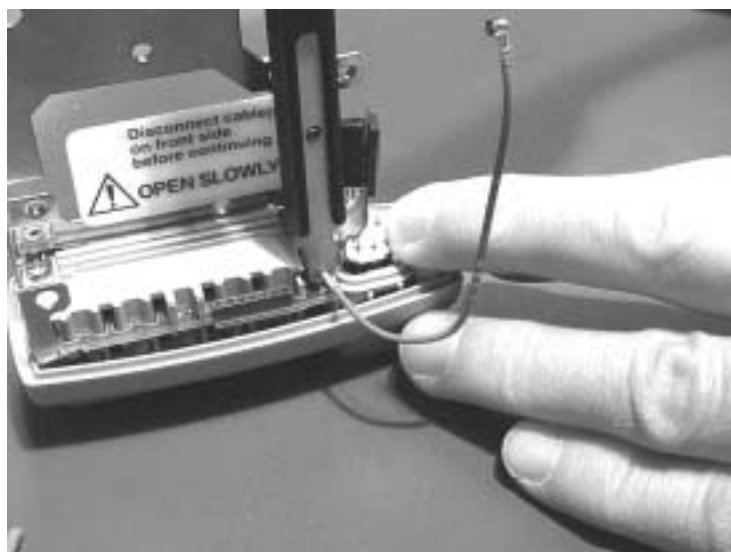
Figure 5-16 Disconnect the RF Cable from the Front End Assembly
