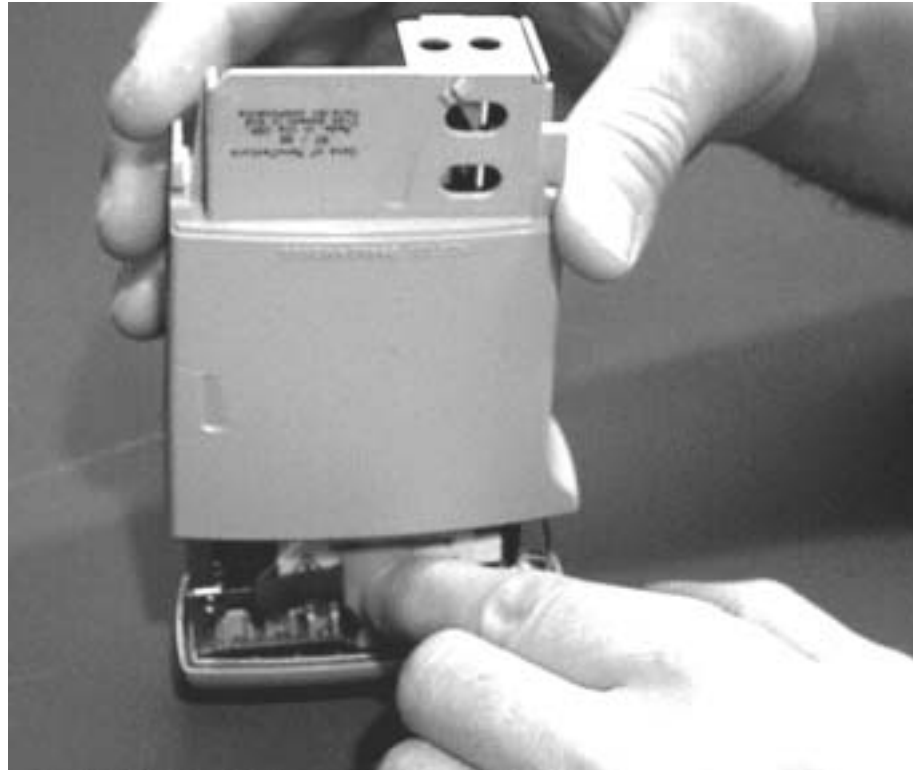
Figure 6-20 Press and Hold the red flex Connector
