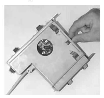
Disconnect pneumatic hose from pump assembly to Main Board secondary pressure transducer on revision 06 units. (Disconnect pressure sensor cable on earlier revisions) The boards can now be slid together up and out of the pcb guides built into the metalwork of the chassis.
