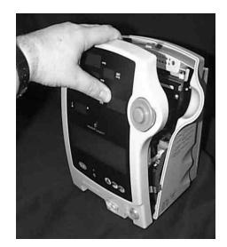
Before the panel can be separated from the case, it is necessary to disconnect the switchboard cable, temperature probe cable and  $SpO_2$  sensor cable if fitted.
