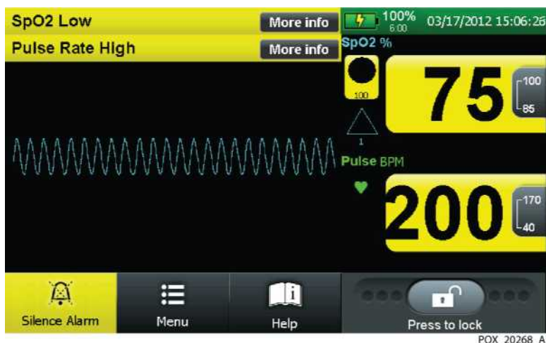
Figure 10-16. LIGHT Test: BPM 200, SpO2 75, MOD low, Light High
