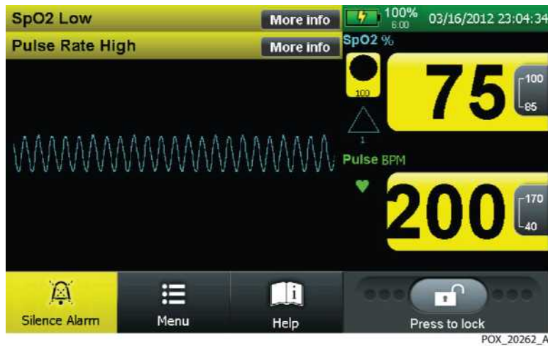
Figure 10-7. BPM Test: BPM 200 and SpO2 75
