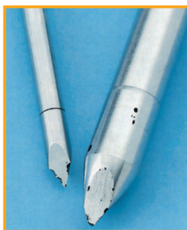
Pitting corrosion on a trocar Cause: High chloride content in the water
