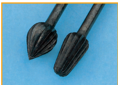
Corrosion on burs Cause: Reprocessing of disposable instruments
