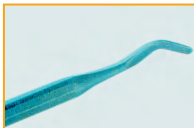
Corroded filling spatula Cause: material attacked by acidic cement remover
