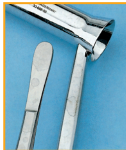
Water stains on an instrument
