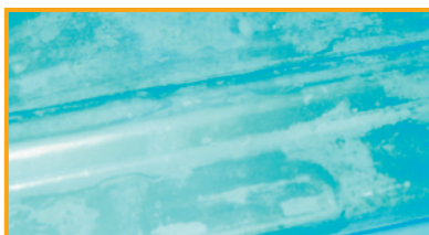
attacked Eloxal (anodized aluminum)
