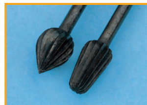
Corrosion on burrs Cause: Reprocessing of disposable instruments
