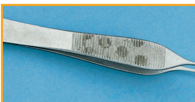
Stains on the tweezers Cause: Insufficient steam quality
