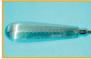
Stained instruments Cause: Drying water
