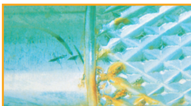
Lime and foreign rust on tooth forceps
