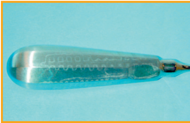
Stained instruments Cause: Drying water with high salt content
