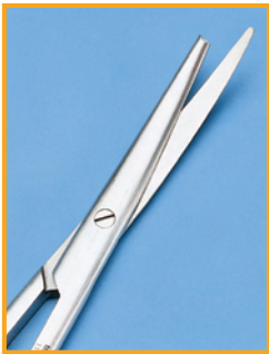
Scissors with broken tip. Cause: wrong handling (instrument was dropped)
