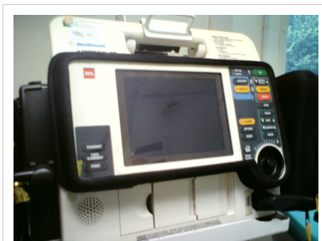
A Lifepak semi-automatic defibrillator/ECG monitor mounted in an ambulance. These units are designed for use only by healthcare professionals and are capable of measuring blood pressure and blood oxygen saturation in addition to the primary functions
