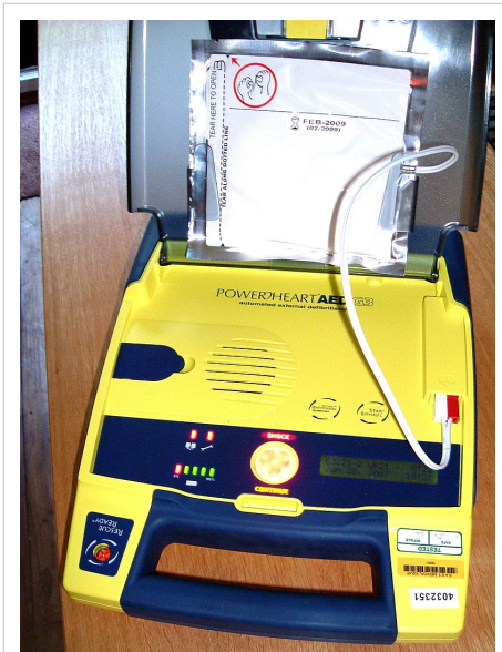
An automated external defibrillator, open and ready for pads to be attached
