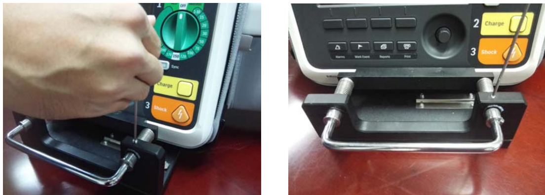
Figure 17 DFM100 Device Installation-6
