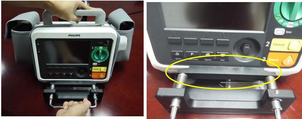
Figure 16 DFM100 Device Installation-5
