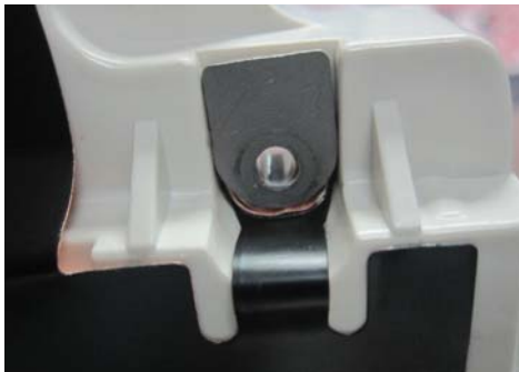
Figure 116 NBP Module Install-4
