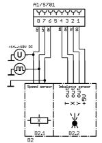
During centrifugation the speedometer pulses of the speed sensor (B2.1) at the bottom of the motor are interrupted.
