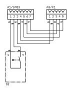
Position switch "Mo" of the motor-driven lid lock closes during the centrifugation run.
