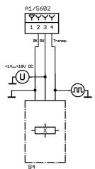
After start-up no speedometer pulses will be received from the speed sensor (B4) on top of the motor.
