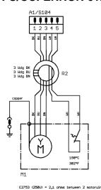
Overtemperature in the motor. Temperature > 150°C / 302°F.
