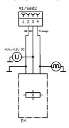
During centrifugation the speedometer pulses of the speed sensor (B4) on top of the motor are interrupted.
