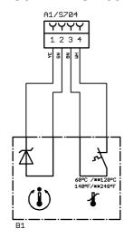
The temperature in the centrifuge chamber measured by the temperature sensor (B1) is out of the valid range.
