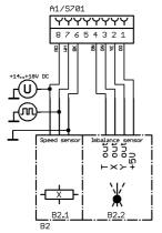
The frequency converter recognises excess speed. It evaluates the signals from the speed sensor (B2.1) at the bottom of the motor.
