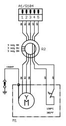
E2753 (250U) = 2,1 ohms between 2 motoruires at cold motor ca. +15...30°C
