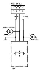
After start-up no speedometer pulses will be received from both speed sensors.
