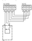
Position switch "Mc" of the motor-driven lid lock opens during the centrifugation run.
