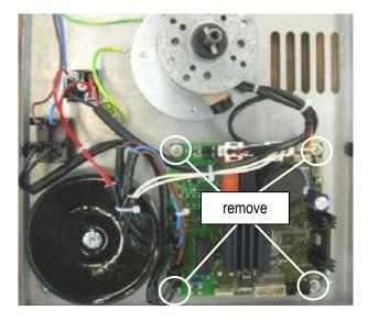
• Put in the new control board, connect all electrical contacts and re-assemble the unit in reverse order.
