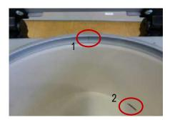
• When mounting the rotor chamber make sure that the ventilation drilling behind on the right points to the corner of the housing (2).
