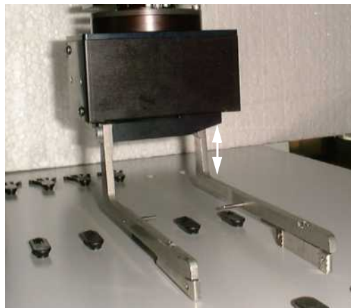
Fig. 8-72 Adjustment of the right gripper finger
