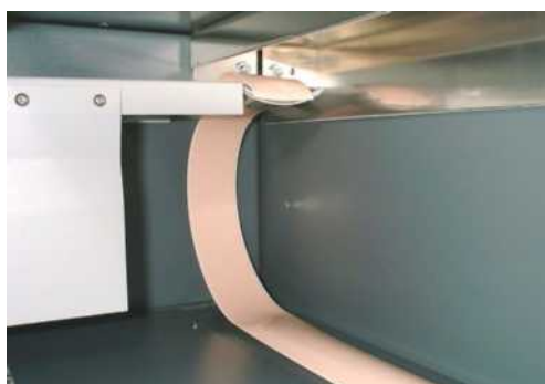
Fig. 8-118 How the flex cable is fixed to the arm
