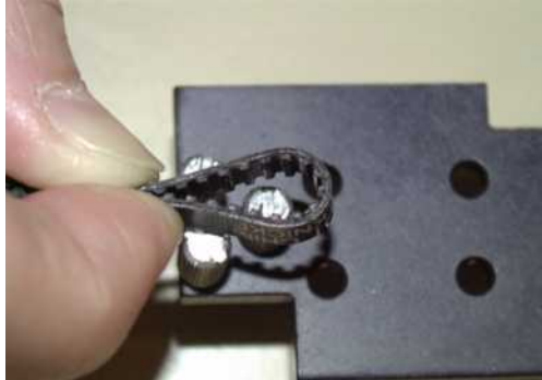
Fig. 8-139 Y-belt connection to the gripper assembly
