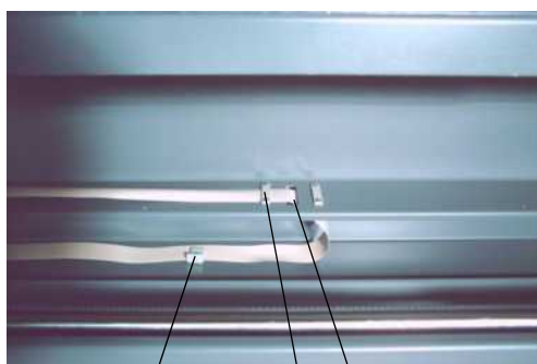
Fig. 8-119 How the flex cable is fixed to the base unit
