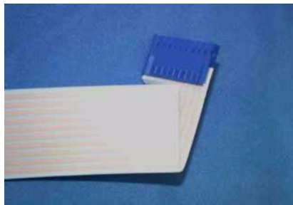
Fig. 8-79 Prepared gripper/rotator flex cable
