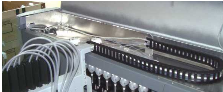
Fig. 8-171 Cable holder chain for tubings and LiHa cable
