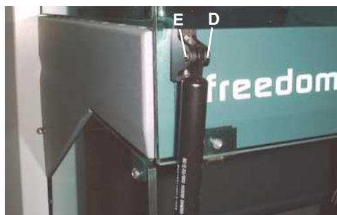
Fig. 8-5 Gas spring fixing flap side
