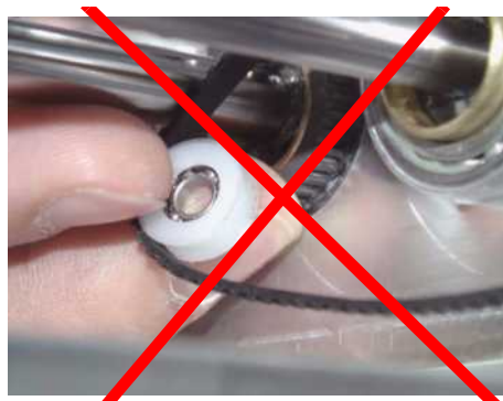
Fig. 8-110 False deflection roller orientation - bearing partly covered
