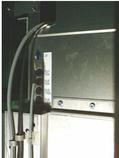
Fig. 8-13 Fuses of power supply module
